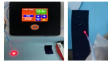
Fig. 9- a - Laser initiation settings and beam profile. b - carbon paper initiation
